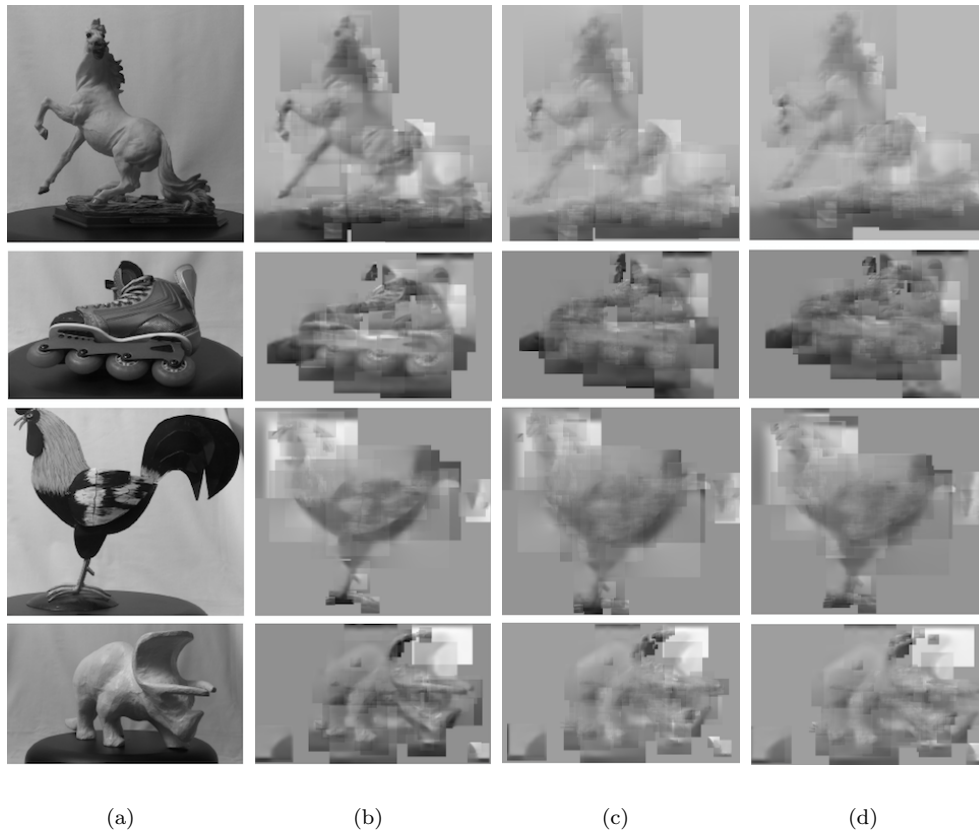
Figure 2.10: Images reconstructed from dense DSP-SIFT. Each pair shows the original and the reconstructed images from dense DSP-SIFT.
